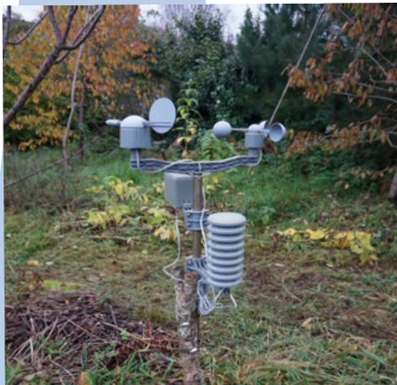
An anemometer for measuring wind speed in the forest garden will help the forest garden see the effect of his design.
